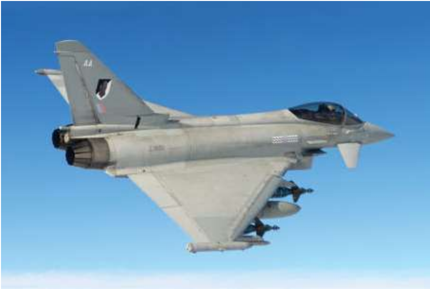
This view of a Royal Air Force Typhoon provides a clear view of the two Towed Radar Decoy dispensers housed in the starboard wingtip pod. ROYAL AIR FORCE/CROWN COPYRIGHT
